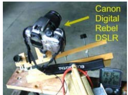
Looking down the Haig mount hinge axis at the hinge/alignment scope (left), camera (above and left of center) and knife-edge/screw (right).
