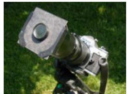
Grating mounted as an "objective" in front of 205-mm telephoto lens
